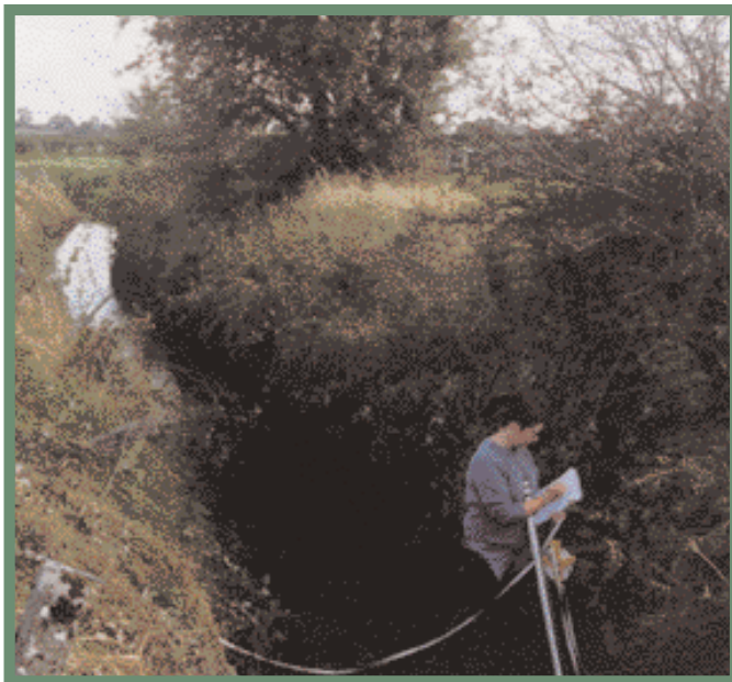
Recording channel width to estimate area
